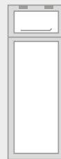
GLASS TO GROUND WINDOW NARROW WITH TOP LITE WIDTH- 537MM HEIGHT- 1755MM WCT10 TOP HUNG TOP LITE
