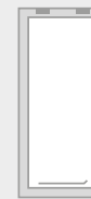
3/4 LENGTH WINDOW NARROW WITH SASH WIDTH- 537MM HEIGHT- 1375MM WCS8 TOP & SIDE HUNG
