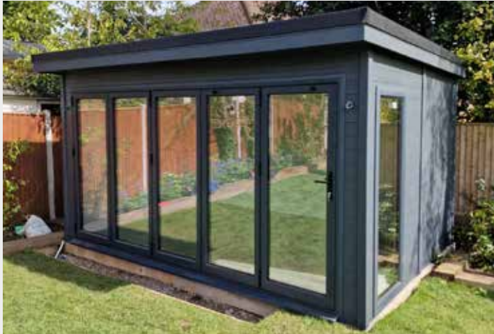
14' X 10' Pent garden studio, thermowood cladding, Aluminium 5 leaf 14ft bifold doors anthracite grey, 1 full length window 710 x 1857, MDF (V grooved) painted lining (white) with breathable membrane (moisture barrier) and Celotex insulation, painted finish in anthracite grey, EPDM rubber roof, laminate floor dark grey oak, oak & black guttering
