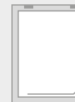
HALF LENGTH WINDOW WIDE WITH SASH WIDTH- 745MM HEIGHT- 1060MM WCS9 TOP HUNG ONLY
