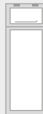
GLASS TO GROUND WINDOW NARROW WITH TOP LITE WIDTH- 537MM HEIGHT- 1755MM WCT10 TOP HUNG TOP LITE
