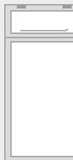
GLASS TO GROUND WINDOW WIDE WITH TOP LITE WIDTH- 745MM HEIGHT- 1755MM WCT15 TOP HUNG TOP LITE
