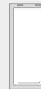
3/4 LENGTH WINDOW NARROW WITH SASH WIDTH- 537MM HEIGHT- 1375MM WCS8 TOP & SIDE HUNG
