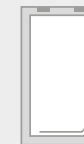
HALF LENGTH GROUND WINDOW NARROW WITH SASH WIDTH- 537MM HEIGHT- 1060MM WCS6 TOP & SIDE HUNG
